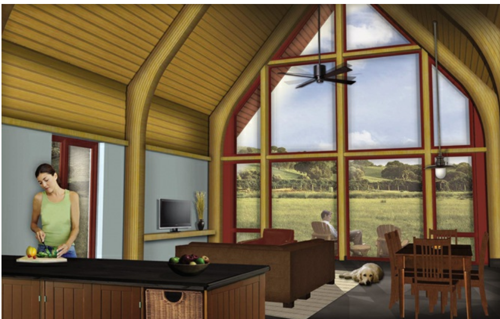
ENERGY SAVINGS ARE ENHANCED BY THE USE OF TRIPLE-PANED WINDOWS COATED WITH THERMAL BREAK FILM, ALONG WITH A CATHEDRAL CEILING TO MAXIMIZE SOLAR GAIN IN WINTER
